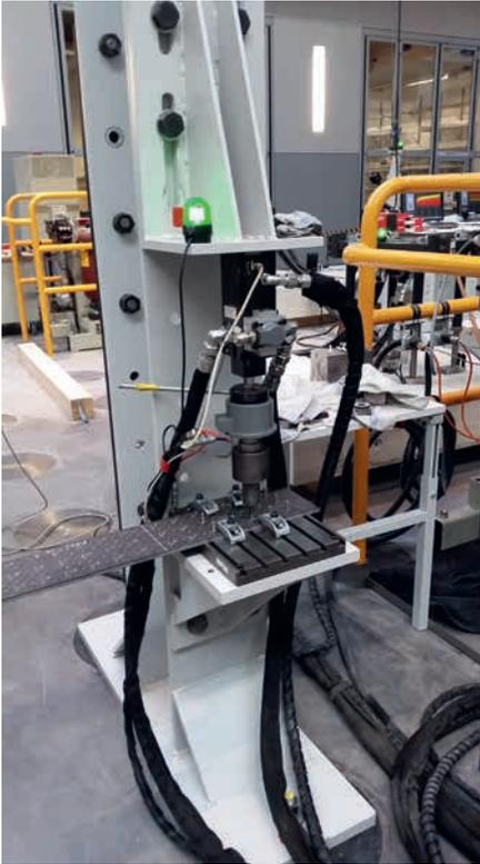
Dynamic tension loading on the new generation X-BT threaded fastener demonstrates excellent robustness of anchorage.
