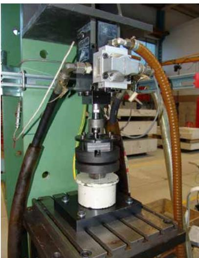
Servo-hydraulic test setup for tension fatigue tests
