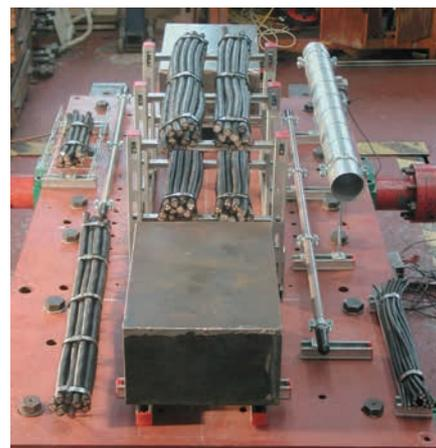
Test configuration: Two base plates were populated with MQ channel fasteners with X-BT studs. The base plates were rigidly attached to the 2-tonne shock loading machine.
