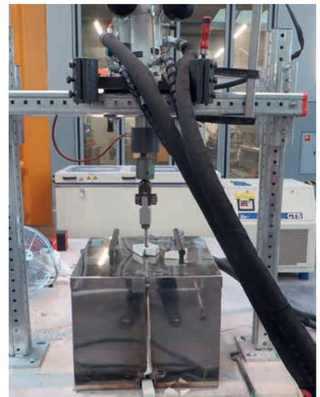
The chamber is heated as long, till the test temperature of the steel base material is reached. The right photo shows the temperature sensor ("black wire") which is fixed in the base material in a small bore hole of 2 mm diameter close to the X-BT threaded fastener. If the target temperature in the base steel is reached, the tension pull-out test is performed (with closed chamber). The photos show the opened chamber after the tension test was executed.
