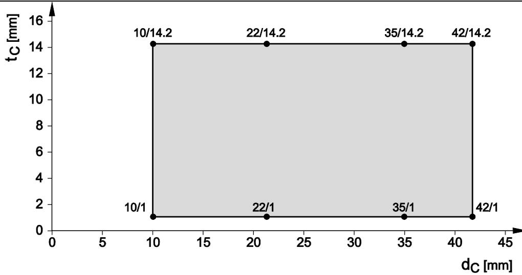
**Copper pipes, floor ( $\geq 150$  mm) – EI 120 / EI 60 / EI 120 plus AP2, C/U**
