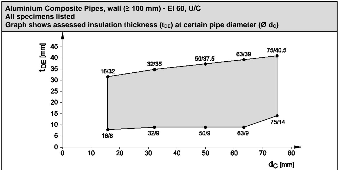
Group 1 of composite pipes (grey shaded) – Brand: Kekelit (Kelox), IVT (Prineto Stabil Rohr), Rehau ( $\leq 40$  mm; Rautitan stabil), TECEflex
