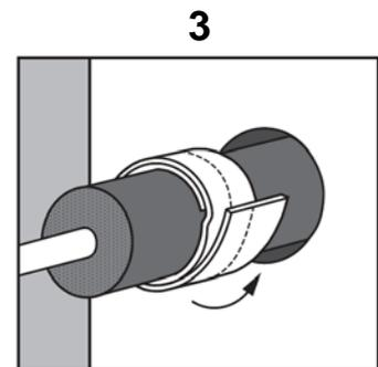
Wrap Hilti Firestop Bandage CFS-B around the insulation. Secure the bandage with steel bands or wire ( $\geq 0,7$  mm)
