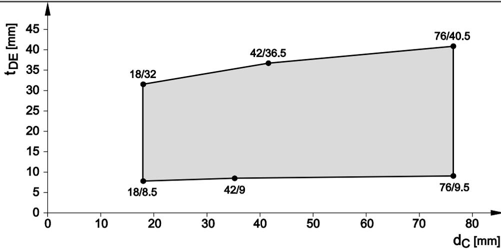
**Steel pipes, wall ( $\geq 100$  mm) – EI 120, C/U plus beading (AP3)
