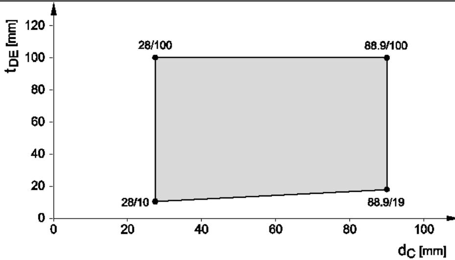
**C.2.1.2.2 Copper pipes with preinstalled Wicu Flex PE Insulation**
