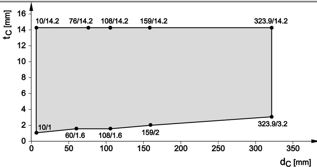
**Steel pipes, floor ( $\geq 150$  mm) – EI 120 / EI 90 / EI 60, C/U**
