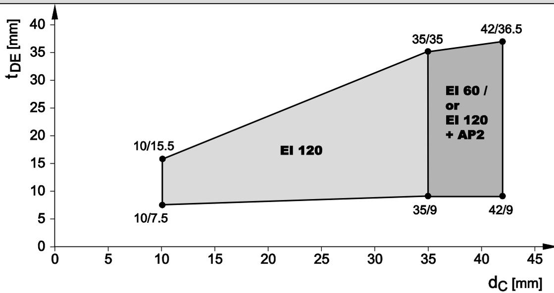
**Copper pipes (Ø 28 - 88,9), floor (≥ 150 mm) – EI 90 C/U**
