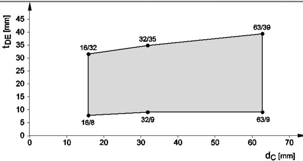
**Plastic pipes PE-HD according EN 12201-2, floor ( $\geq 150$  mm) - EI 180, U/C**
