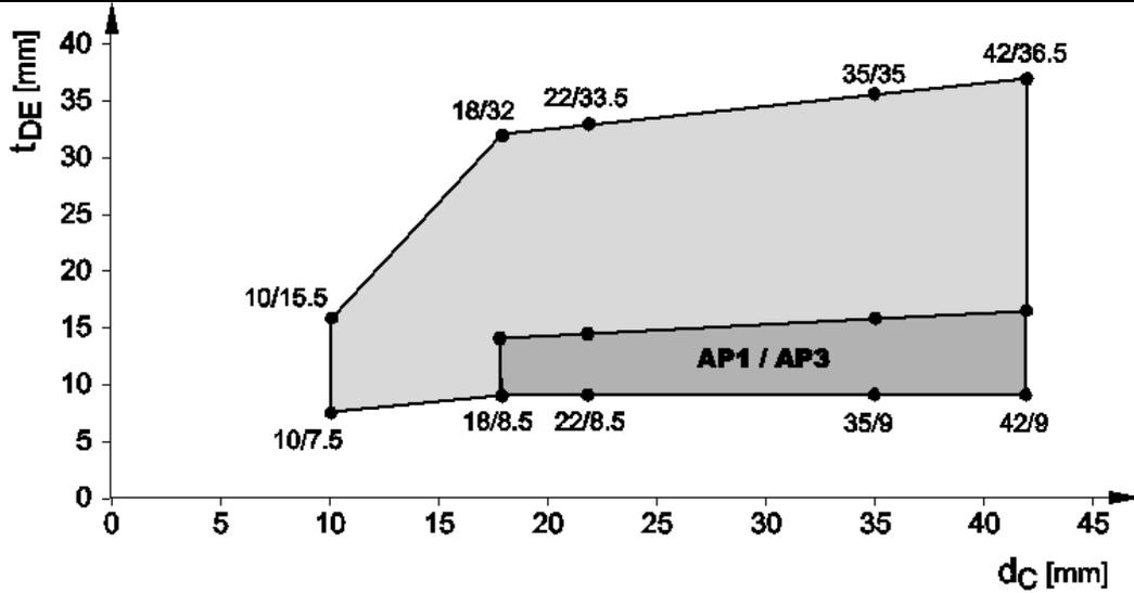
**Copper pipes, wall ( $\geq 100$  mm) – EI 120, C/U plus AP3**
