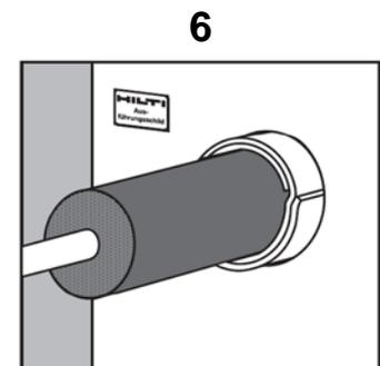
If it is necessary, an additional insulation over the bandage has to be installed.
