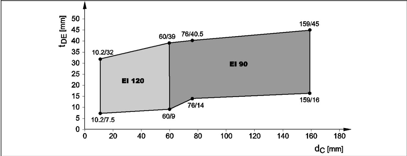
**Steel pipes, rigid wall ( $\geq 200$  mm) – EI 120, C/U**
