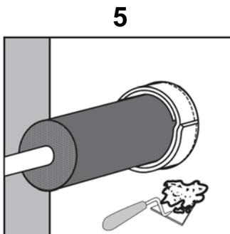
Close the remaining gap with mortar or gypsum.
