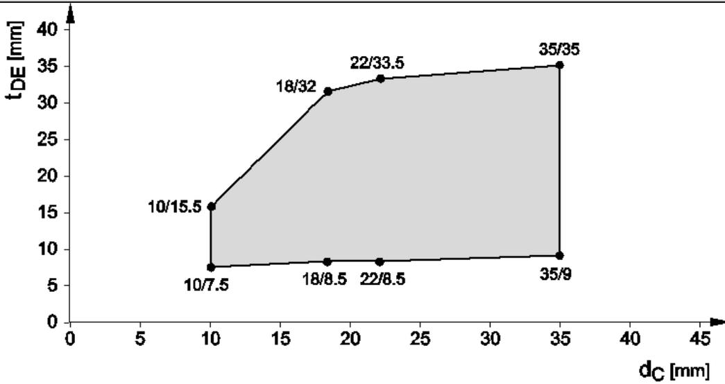
**Copper pipes (Ø 28- 88,9), wall (≥ 100 mm) – EI 90 C/U**
