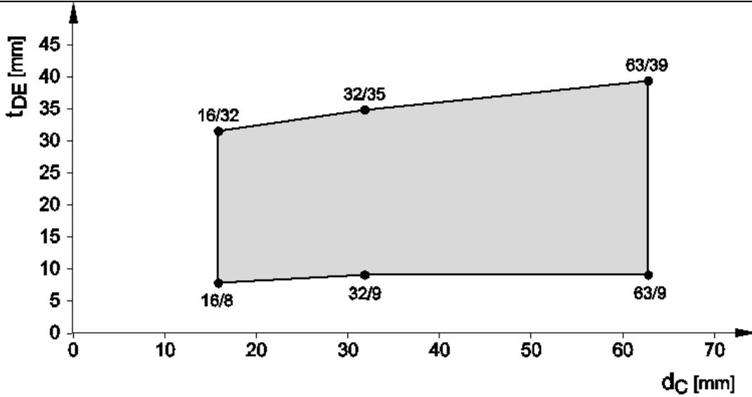
**Plastic pipes PE-HD according EN 12201-2, wall ( $\geq 100$  mm) - EI 120, U/C**
