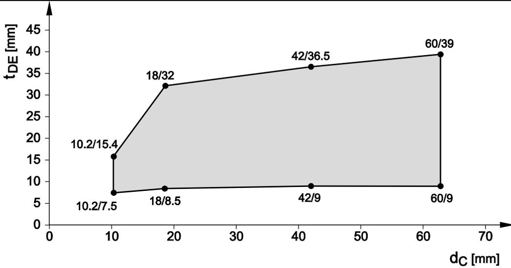
**Steel pipes, walls ( $\geq 100$  mm) – EI 90 with AP1, C/U
