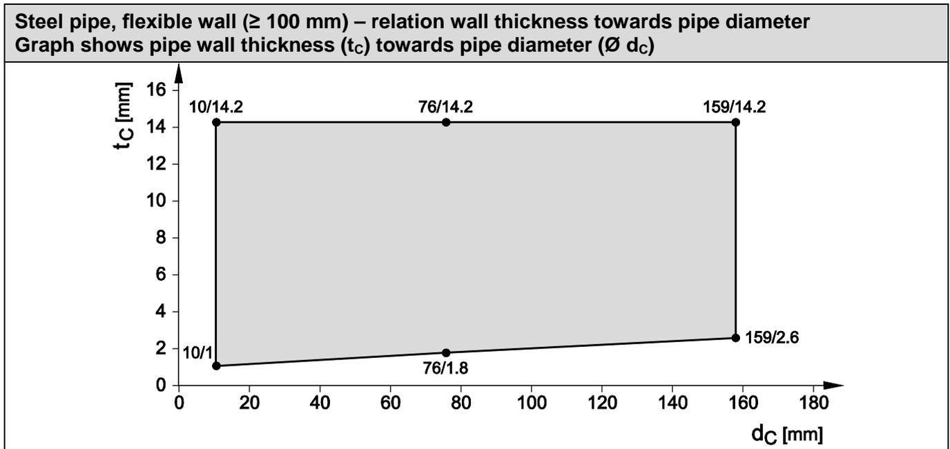
**Steel pipes, flexible wall ( $\geq 100$  mm) – EI 90 / EI 120 (dotted line) C/U**
