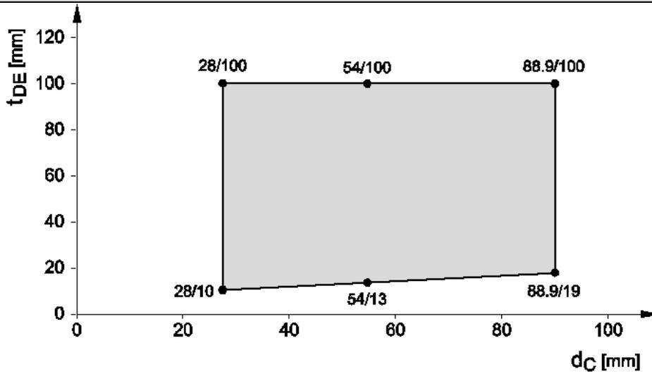
**C.2.3.2.2 Copper pipes with preinstalled Wicu Flex PE Insulation**
