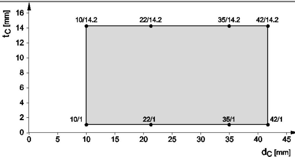
**Copper pipes, wall ( $\geq 100$  mm) – EI 90, C/U (plus AP1 or AP3)**
