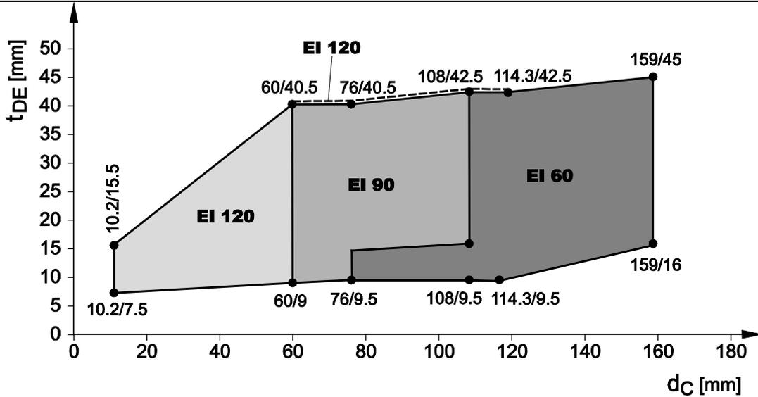
**Steel pipes, floor ( $\geq 150$  mm) – EI 120, C/U plus AP2**
