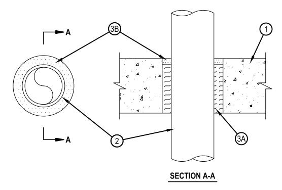
1. Floor or Wall Assembly — Min 4-1/2 in. (114 mm) thick reinforced lightweight or normal weight (100-150 pcf or 1600-2400 kg/m3) concrete floor or 5 in. (127 mm) thick reinforced lightweight or normal weight concrete wall. Floor/wall may also be constructed of any UL Classified Concrete Blocks\*. Max diameter of opening is 5 in. (127 mm).
