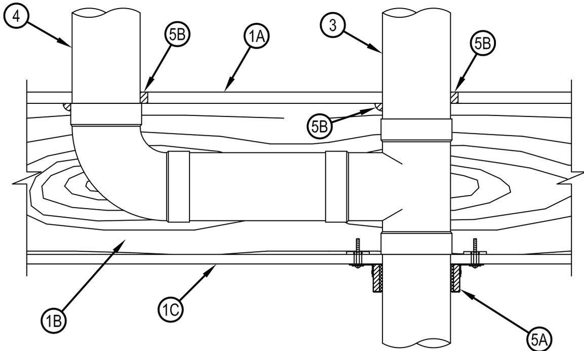
1. Floor-Ceiling Assembly — The 1 hr fire-rated solid or trussed lumber joist floor-ceiling assembly shall be constructed of the materials and in the manner specified in the individual L500 Series Floor-Ceiling Designs in the UL Fire Resistance Directory. The general construction features of the floor-ceiling assembly are summarized below:
