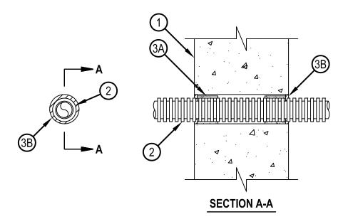
1. Wall Assembly — Min 6-1/2 in. (165 mm) and 7-1/2 (191 mm) thick reinforced lightweight or normal weight (100-150 pcf or 1600-2400 kg/m3) concrete for 3 and 4 hr fire rated wall assemblies, respectively. Wall may also be constructed of any UL Classified Concrete Blocks\*. Max diam of opening is 3 in. (76 mm).
