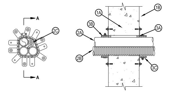
1. Wall Assembly — Min 6 in. (152 mm) thick reinforced lightweight or normal weight (100-150 pcf or 1600-2400 kg/m3) concrete. Wall may also be constructed of any UL Classified Concrete Blocks\*. Max diam of opening is 4 in. (102 mm).
