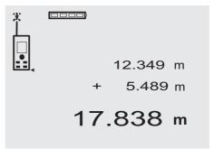
Individual distances can be conveniently added. This is useful, for example, for determining the total length of
