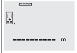
Press the "Measure" button once. The laser beam is switched on and is visible in the form of a spot on the target surface. This aiming mode is indicated in the display by a blinking laser symbol.
