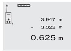
Individual distances can be conveniently subtracted from each other, e.g. in order to determine the distance between the underside of a pipe and the ceiling. This can be done by subtracting the distance between the floor and the underside of the pipe from the distance between the floor and the ceiling. If the pipe diameter is subtracted, the result is the distance between the top of the pipe and the ceiling.
